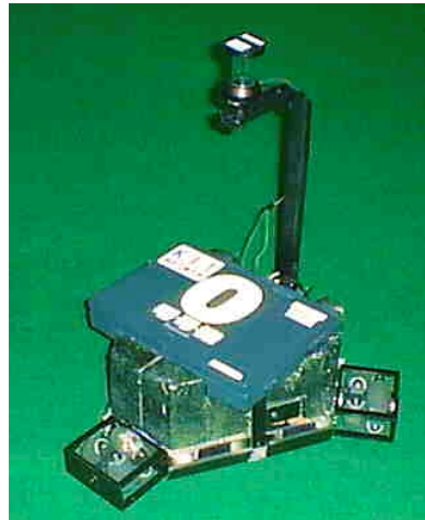
Fig. 2. Prototype of the Omnidirectional Mobile Robot
